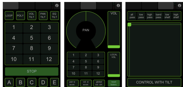
Figure 4. Three iPhone/iTouch layouts control sound file selection, volume/panning, and EQ.
